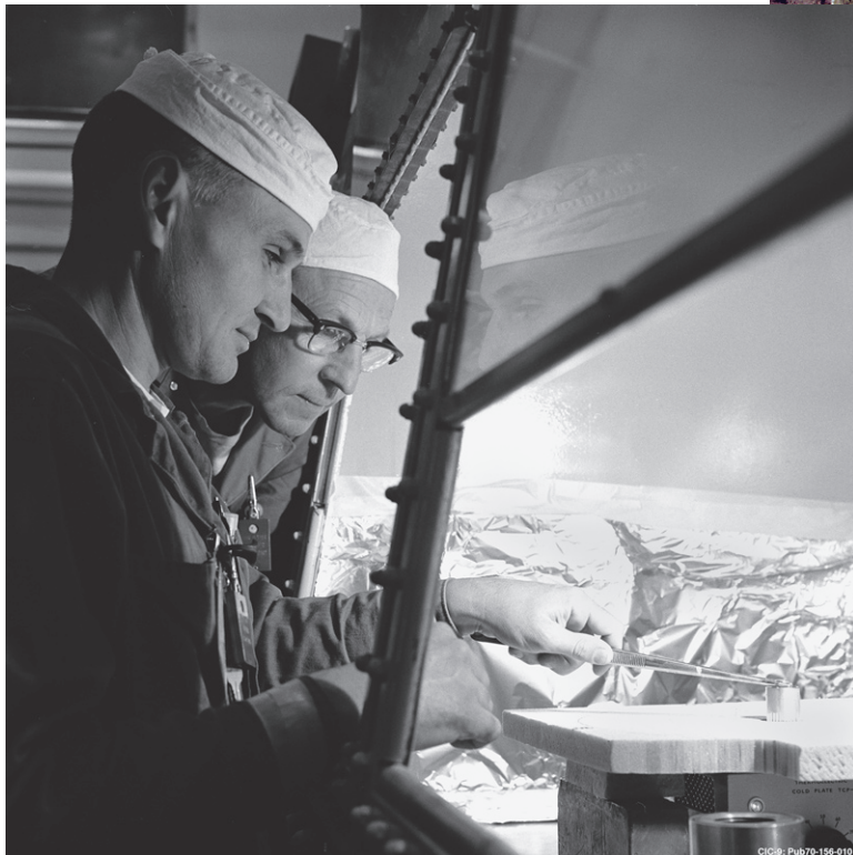
(Left) Workers remove a plutonium-238 heat source from a “target.” (Above) Aerial view of TA-21, DP Site (circa 1979).
